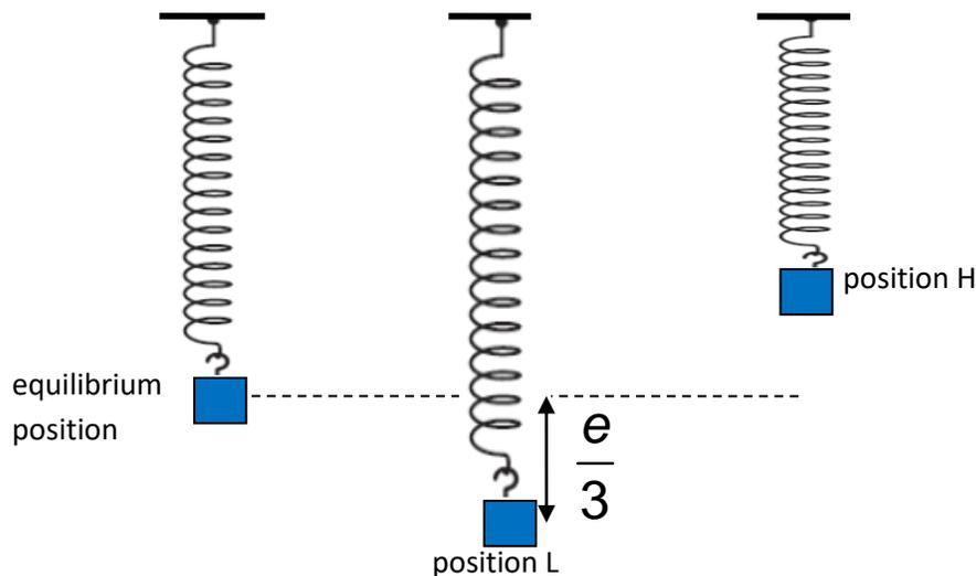
When the mass is released, it performs simple harmonic oscillations between positions L and H with angular frequency  $\omega$ . The displacement from equilibrium is given by the equation
